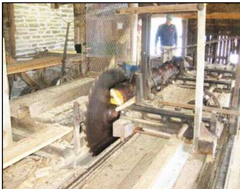
This photo shows a log on the movable carriage being cut by the 48" saw.
