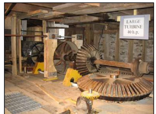
Photo of a large gear on the 40-hp turbine that produces power for the saw.
