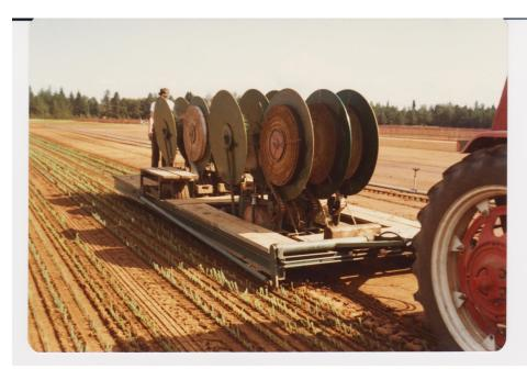
The six-row tape transplanter showing loaded and unloaded reels.
